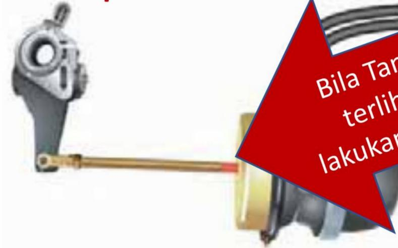
Brake Adjustment-Manual Slack Adjuster
